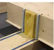
For permanent airtightness of the element joint we offer an airtight sealing cord. It is adhesive on both sides and combines high adhesive power, durability and adaptability. On request, we can interrupt the tongue at the bearing of the element and fill in the groove. The end of the sealing cord has to be pressed onto the bearing on site.
